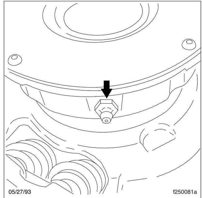
**Fig. 1, Release Bearing Grease Fitting**
