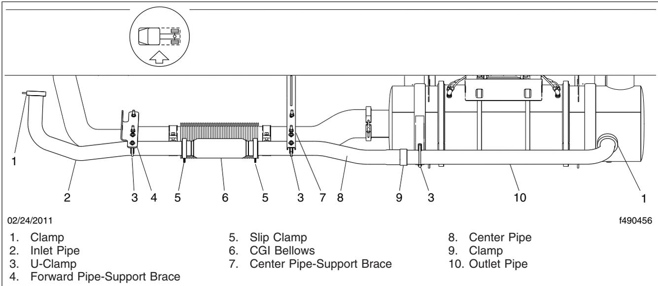
**Fig. 6, CAT EPA07 Exhaust Installation with CGI Bellows**
