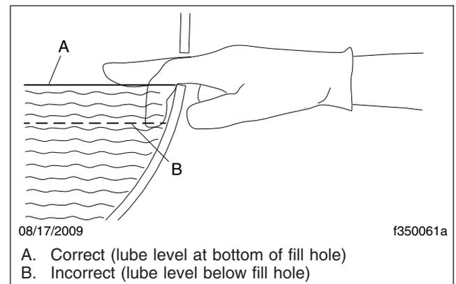
**Fig. 1, Axle Lubricant Level Inspection**
