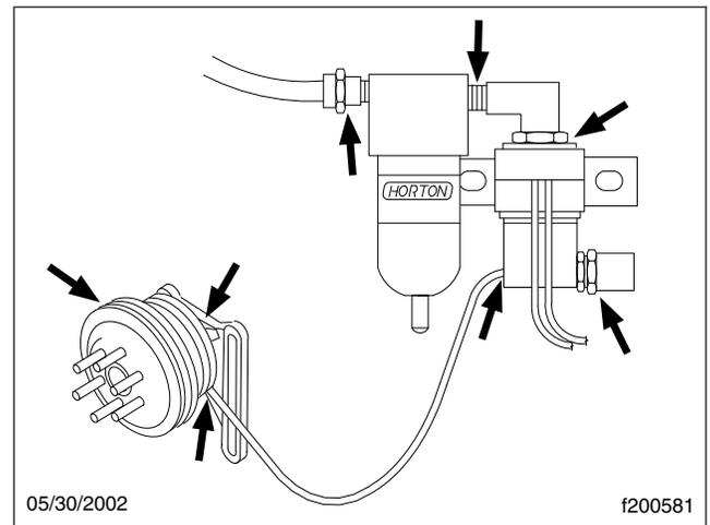
**Fig. 1, Checking for Air Leaks (Horton DriveMaster)**
