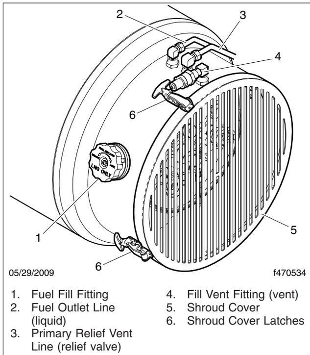
**Fig. 4, Fuel Tank Outer Shell**
