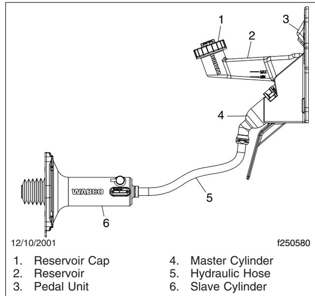
**Fig. 5, Clutch Components**
