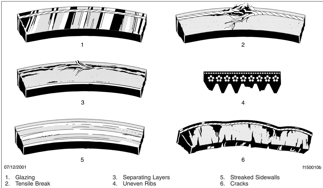
**Fig. 1, Drive Belt Replacement Conditions**
