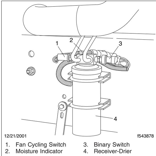
**Fig. 1, Receiver-Drier**
