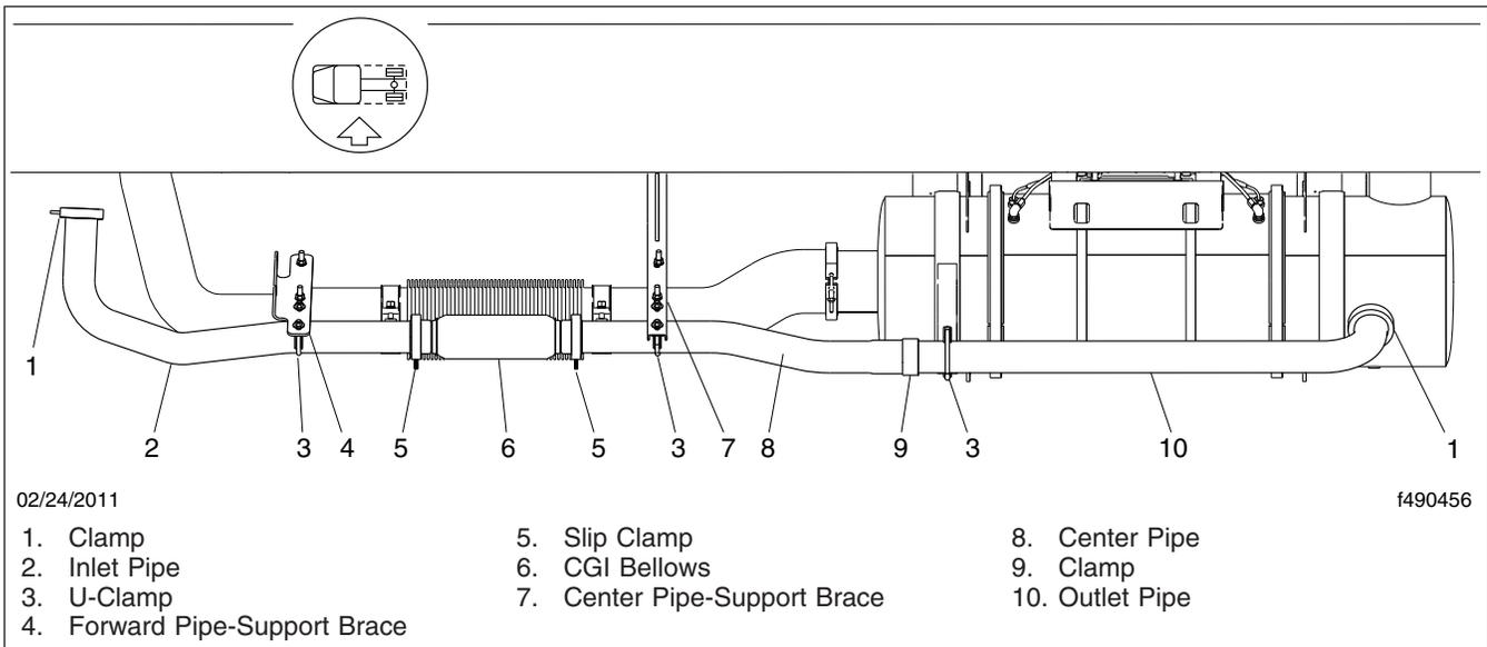
**Fig. 5, CAT EPA07 Exhaust Installation with CGI Bellows**
