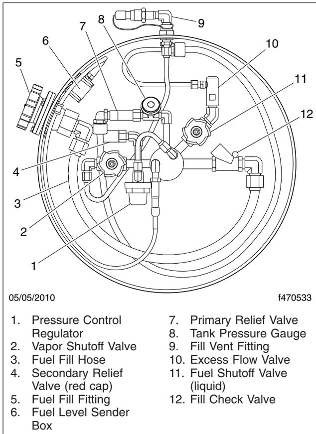
**Fig. 5, Fuel Tank Plumbing Components**
