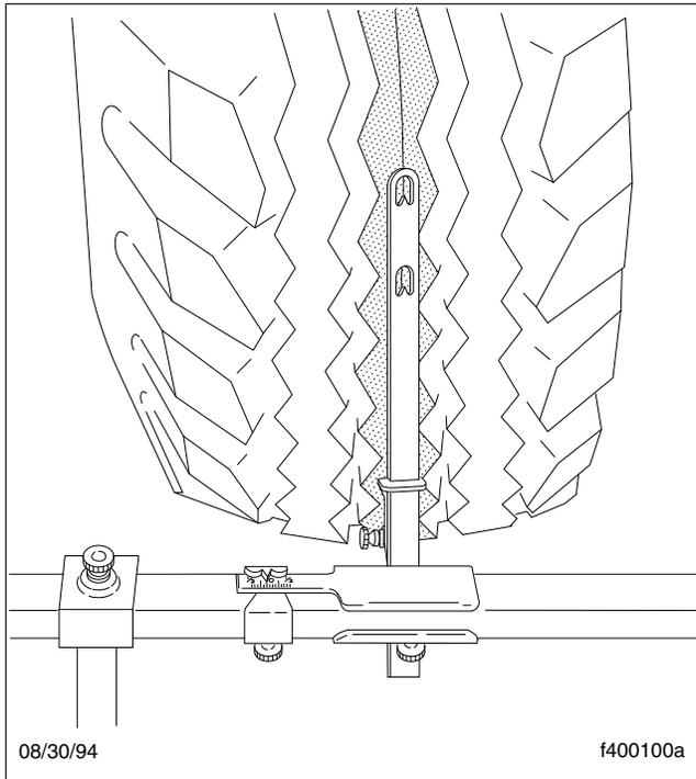
**Fig. 11, Setting Trammel Bar Pointers**
