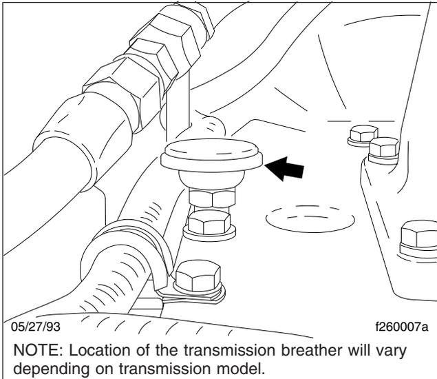
Fig. 3, Transmission Breather (Eaton Fuller shown)
