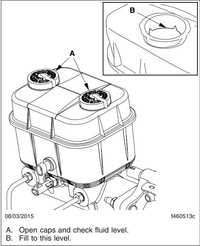
**Fig. 10, Hydraulic Brake Fluid Reservoir (Bosch reservoir shown, Bendix reservoir similar)**
