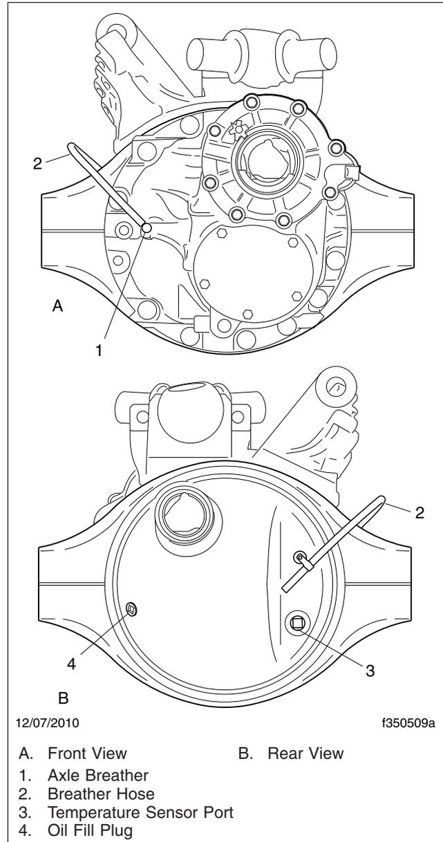
**Fig. 3, Detroit Tandem Axle (forward axle shown)**
