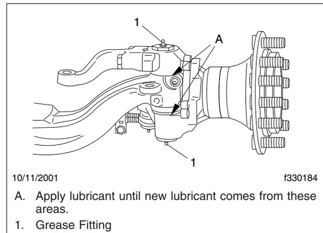
**Fig. 4, Sealed, Easy Steer Plus Kingpin Lubrication**
