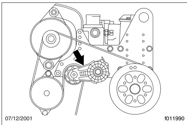
**Fig. 2, Belt Tensioner on Caterpillar 3126 Engine**
