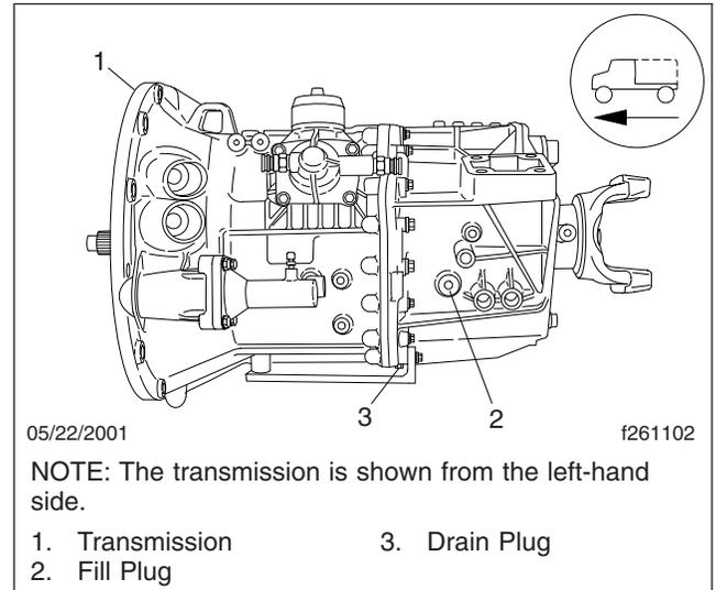
**Fig. 7, Mercedes-Benz Transmission Drain and Fill Plugs**
