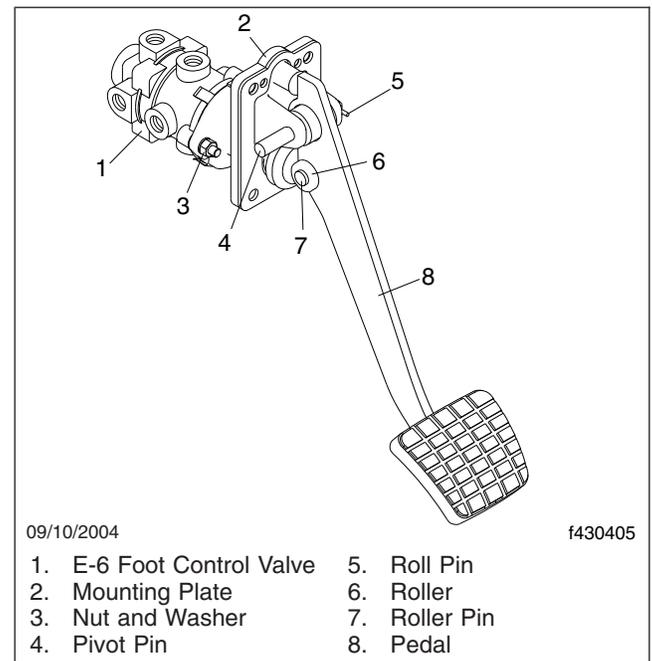
**Fig. 9, Brake Pedal and Valve Assembly**
