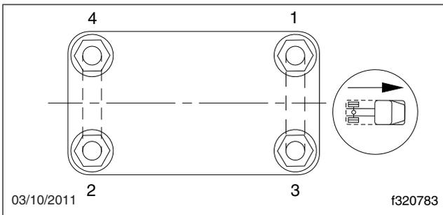
**Fig. 9, Tightening Pattern for U-Bolt High Nuts**
