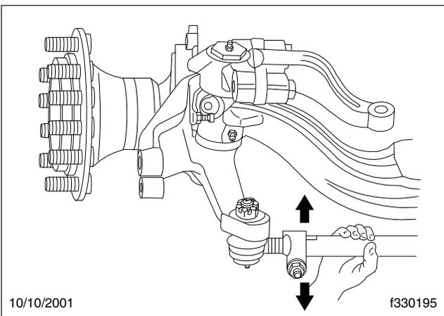
**Fig. 7, Check Movement of Tie Rod End**
