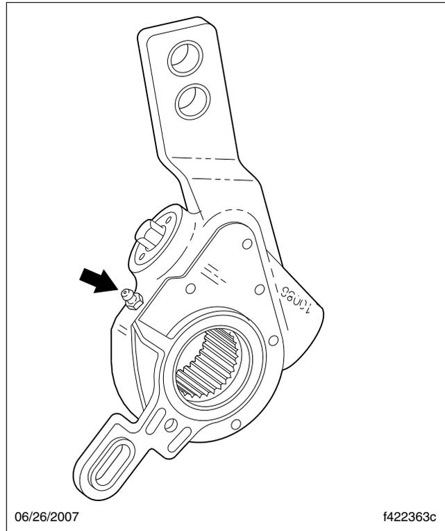
Fig. 5, Haldex Automatic Slack Adjuster Grease Fitting
